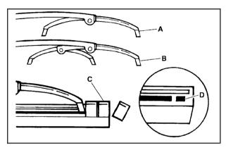
4. To install the new wiper insert, slide the insert (D), notched end last, into the end with two blade claws (A). Slide the insert all the way through the blade claws at the opposite end (B). The plastic caps (C) will be forced off as the insert is fully inserted.
